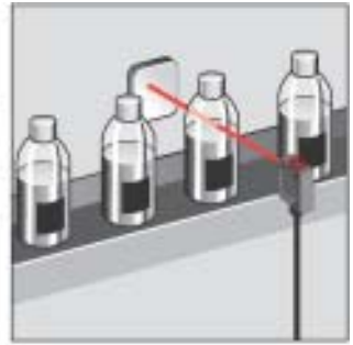
BOS 6K-.../ BOS 21M-... Retroreflective for glass sensing
