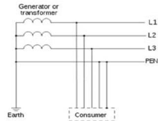
Figure 2: TN-C wiring diagram.
